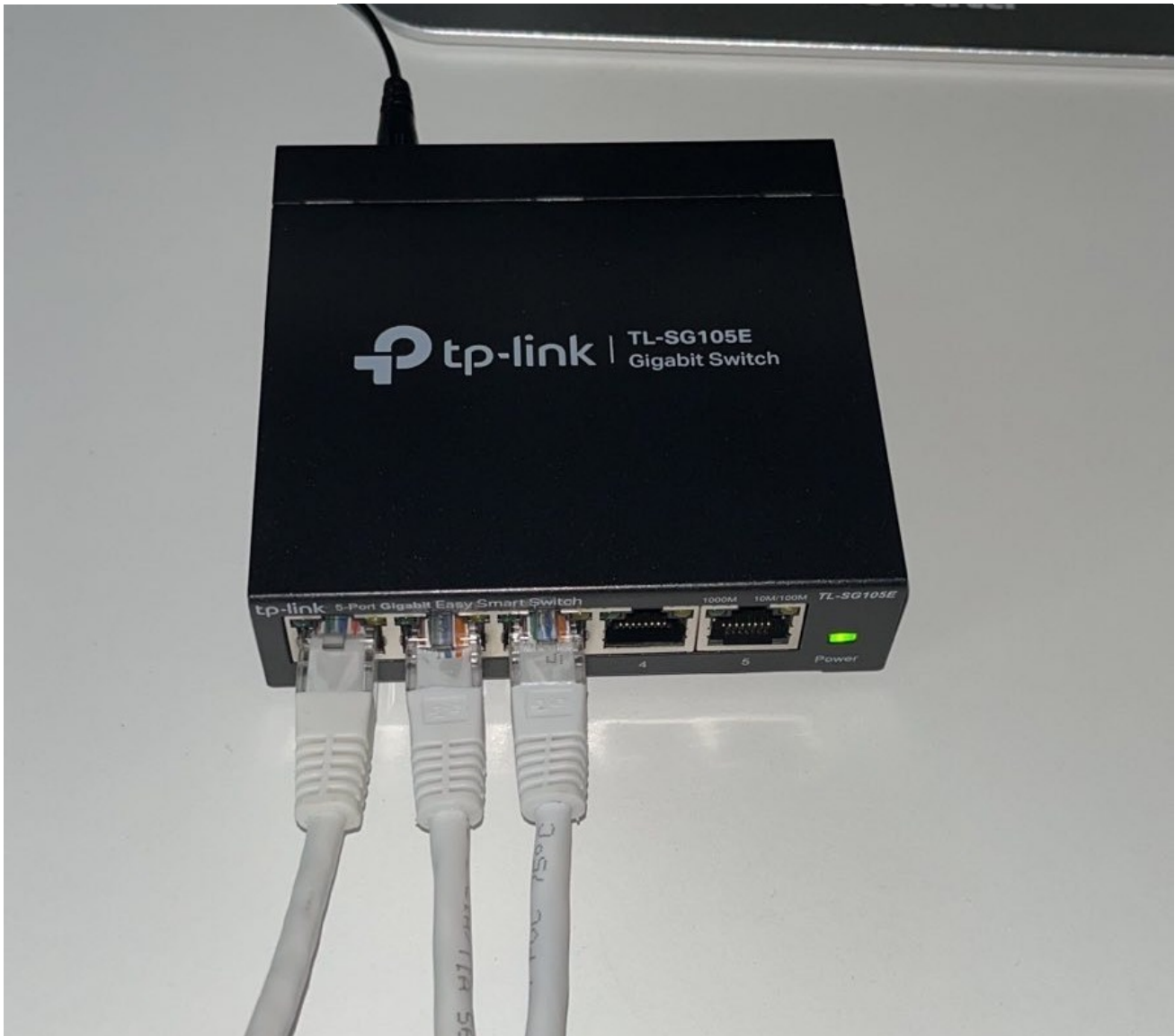
Figure 7 - Non-company switch to network port
